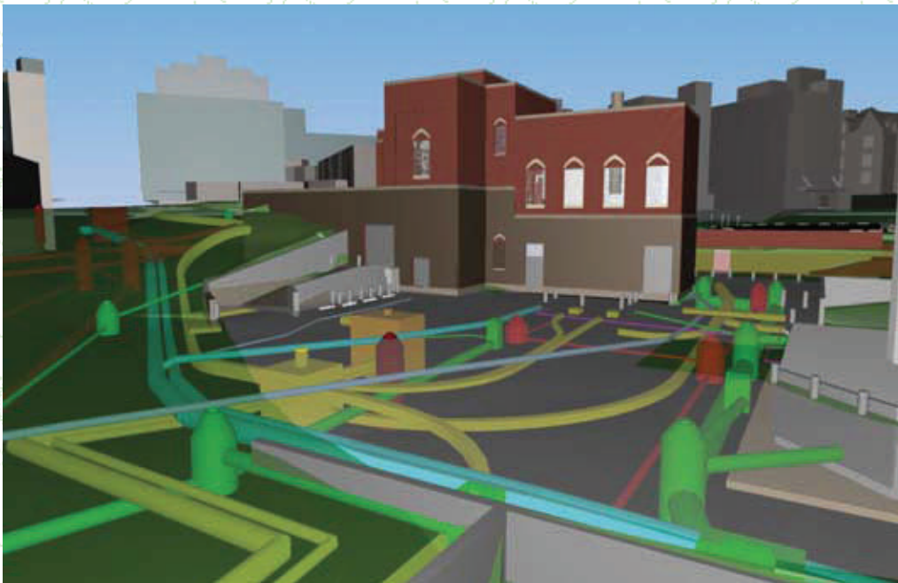
A close-up 3D rendering shows the complex pipe network surrounding the Duke University West Campus Steam Plant.
